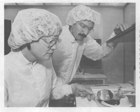
THE PHOTOLITHOGRAPHY ROOM of the PDFL. Elaine Buck (left) and David King (both 6224) demonstrate the application of a layer of photoresist, a processing step that prepares cells for photomasking. Lit by an eery yellow light to which photoresist is insensitive, the room is referred to as the "yellow-light" room.
